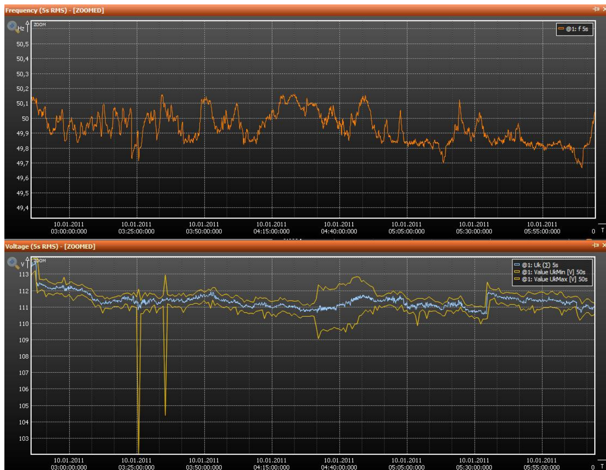
Figure 8: Inconspicuous plot of grid frequency (upper panel) and at the same time some very obvious short time voltage dips and deviations at the same point of measurement (lower panel)
