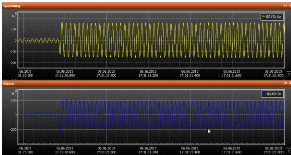
Figure 4: Fault record example U_o and I_o
