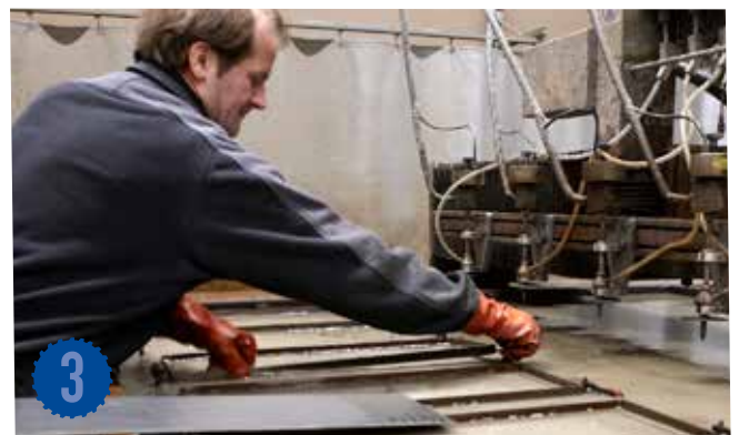
3 Water jet cutting of details.
