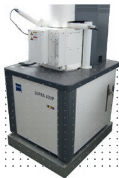
■ Scanning Electron Microscope on Sandwich Platform
