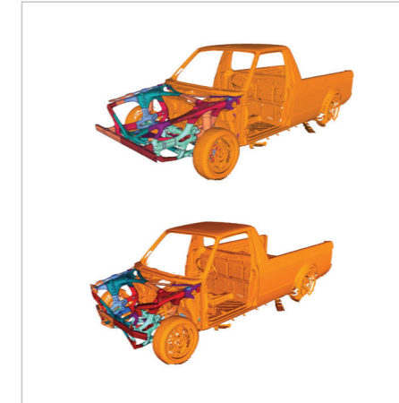
The refined final geometry is subsequently evaluated in an FE analysis.
