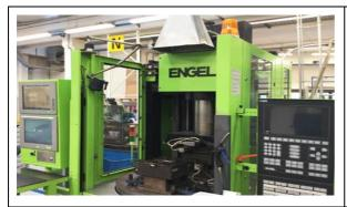
ATAM\_Presses for thermosetting epoxy resin overmoulding, inserted in the IoT system of the company.
