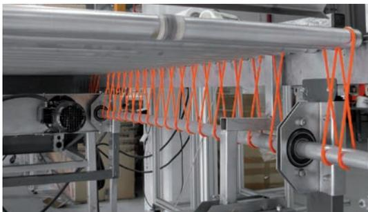
Twisted round belts with hook joint are applicable as live roller drive belts, whereas several belts are installed on on shaft. The mechanical hook joint enables quick and easy assembling. Twisted round belts are available in fabricated length from 250mm to 710mm.
