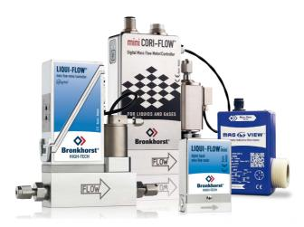
Mass Flow Meters and Controllers for liquids in ranges between 0...75 mg/h and 0...600 kg/h (water equivalent). Our thermal mass flow meters only require a small differential pressure. Despite utilizing direct measurement (i.e. without a by-pass) the temperature rise of the fluid is minimal; only approx. 1...5 °C. This greatly limits the danger of evaporation or degradation of the fluid. The thermal Mass Flow Meters can be close-coupled to a Bronkhorst® control valve for pulsation-free control.
