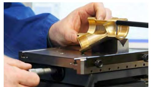
testing with a contourograph
