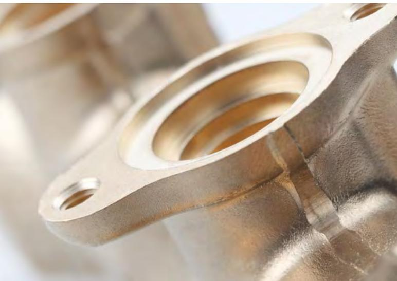
By drop forging (hot forging) in our in-house hot forge full and hollow parts weighing around 5,000 g are created at temperatures that are adjusted to the materials used. Various copper-zinc alloys (brass) as well as low dezincification and modern, lead-free brass alloys are processed in accordance with DIN 50930-6.
