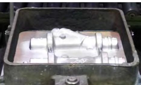
moulding box with valve contour
