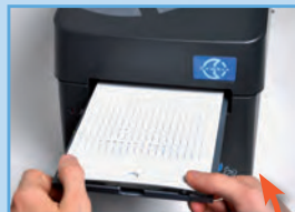
Locate template and media on carriage
