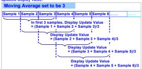
Remark: The higher moving average setting wouldn't cause the response time of Relay and Analogue output slower after first 3
