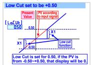
If set the negative value (X2) here to display "X2" which it expressed to be low-cut the PV that it's under the X2 setting value;
