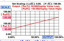
The range between [RoHS] and [RoLS] should be over 20% of span at least; otherwise, it will be got less resolution of analogue output.
