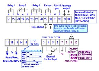
Please check the voltage of power supplied first, and then connect to the specified terminals. It is recommended that power supplied to the meter be protected by a fuse or circuit breaker.
