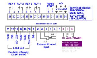
Please check the voltage of power supplied first, and then connect to the specified terminals. It is recommended that power supplied to the meter be protected by a fuse or circuit breaker.
