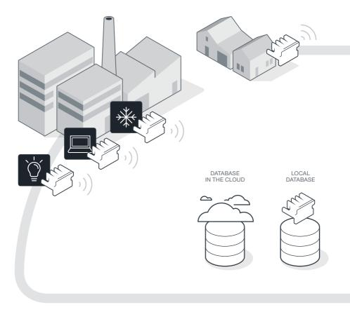
Wibeee logs the installation's electrical parameters so that you can view them from wherever you want: from your office computer, with a smartphone from the local coffee shop or lying down on your sofa at home with your tablet. Wibeee can also work in tandem with any other device that is compatible with the PowerStudio SCADA system.
