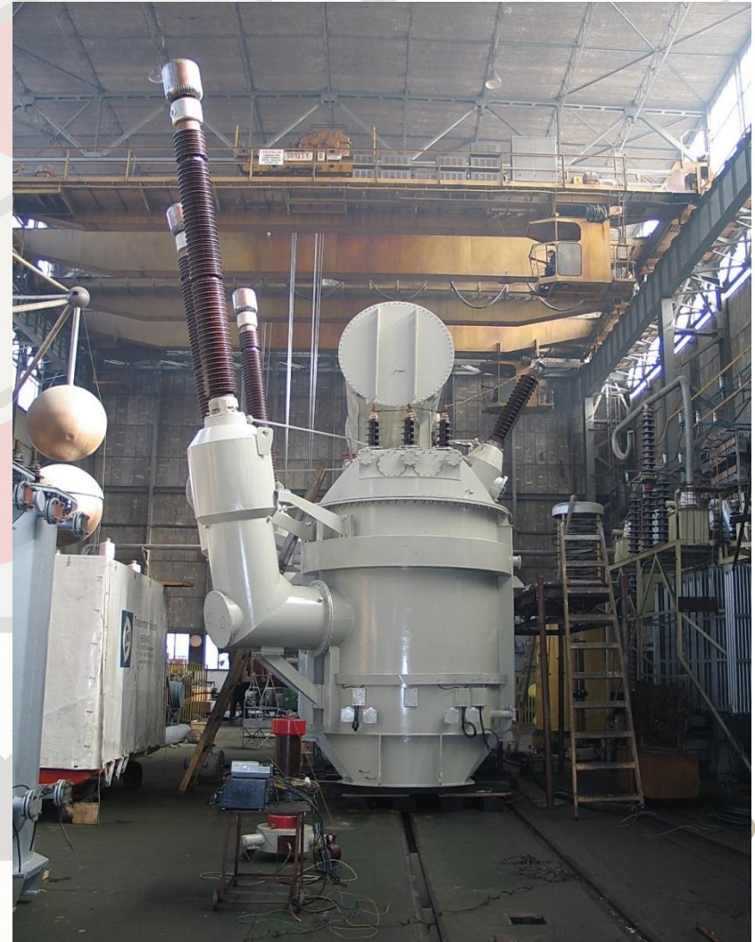
Power transformers 90 MVA, city Harare - Zimbabwe
