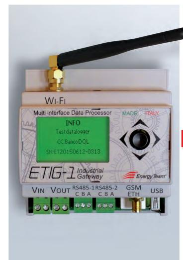
ETIG-1 is ideal for acquiring and filing data from instruments measuring electricity, gas, water, steam, heat, ect. it then sends all the collected measurements to one or more servers for data publication.
