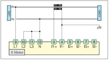
Direct insertion in a Three-phase electrical network BT, with neutral wire
