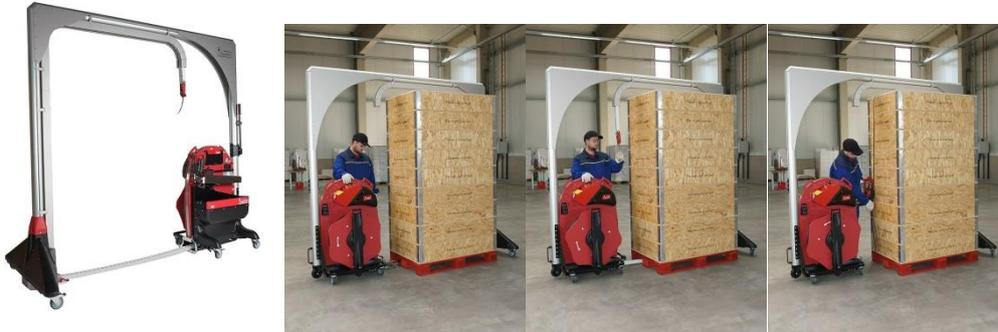
This additional device enables the strapping of pallets up to 3.00 m in height. It is also ideally suitable for the reliable and careful strapping of projecting packages or pallets containing sensitive goods (such as painted surfaces).
