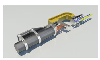
The joining gun bonds metal and plastic in seconds and can be mounted on a robot arm in place of a spot welding gun, for example.
