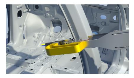
The HPCI technology is used to integrate composite parts to metallic car body structures. © Fraunhofer IWS Dresden
