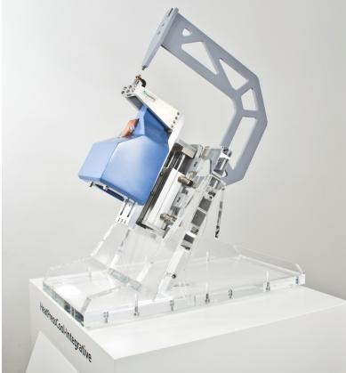
The joining gun presses metal to plastics and simultaneously heats the area by induction.
