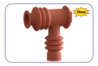
Reusable Insulating Boots are designed to be used with all types of Terminations and is suitable for use with PILC / XLPE Cables. The modified Silicon / Rubber used in shrouds gives the required flexibility and electrical characteristics to ensure sufficient di-electric strength is provided between Phase to Phase and Phase to Ground.
