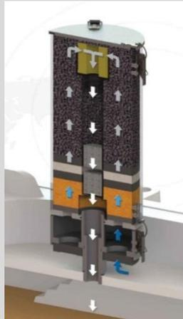
**Objective:** Protecting the environment from contamination with oil mist
