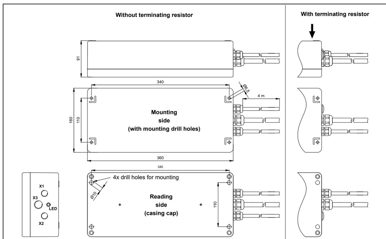
**Figure 9** Outline of antenna HG 98780UA with/without terminating resistor
