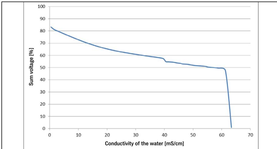
**Figure 33** Attenuation of the sum voltage as a function of the conductivity of the water (30 mm water level)
