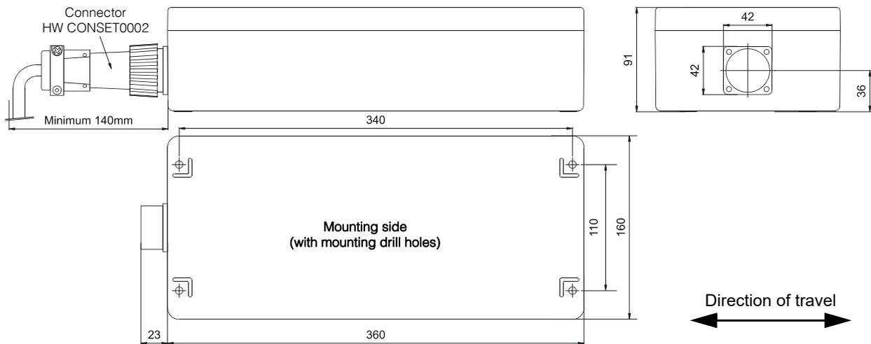
**Figure 7** Outline antenna HG 98780ZA/WA (with casing dimensions)
