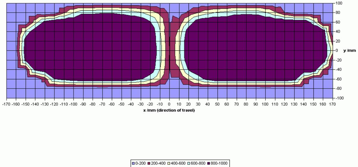
**Figure 25** Diagram 5, Reception voltage X within the antenna area at reading distance 40 mm
