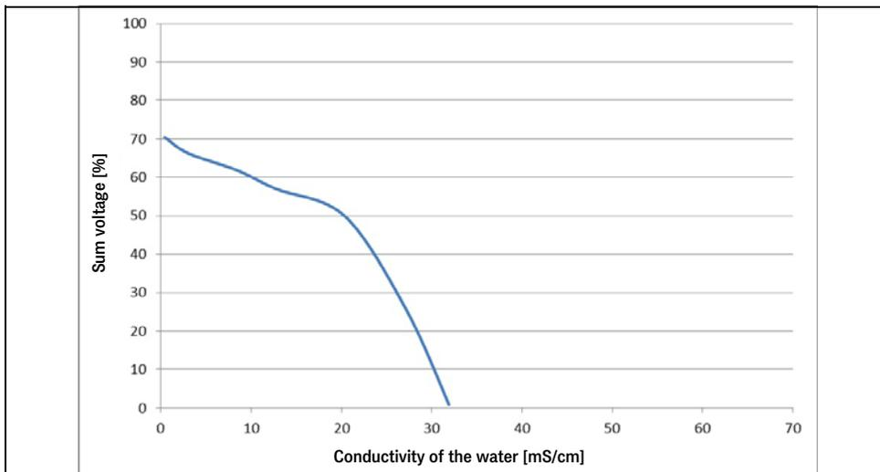
**Figure 34** Attenuation of the sum voltage as a function of the conductivity of the water (75 mm water level)
