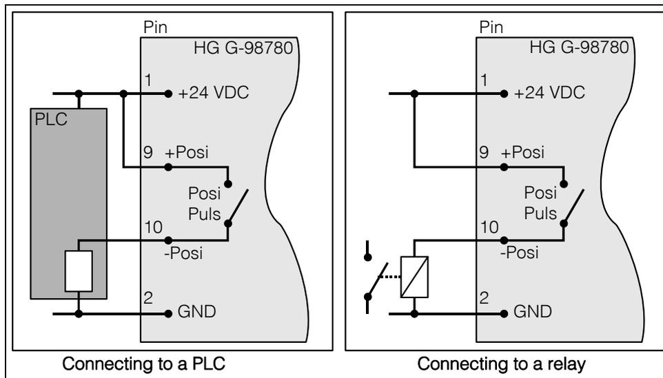
**Figure 10** Connection possibilities positioning pulse
