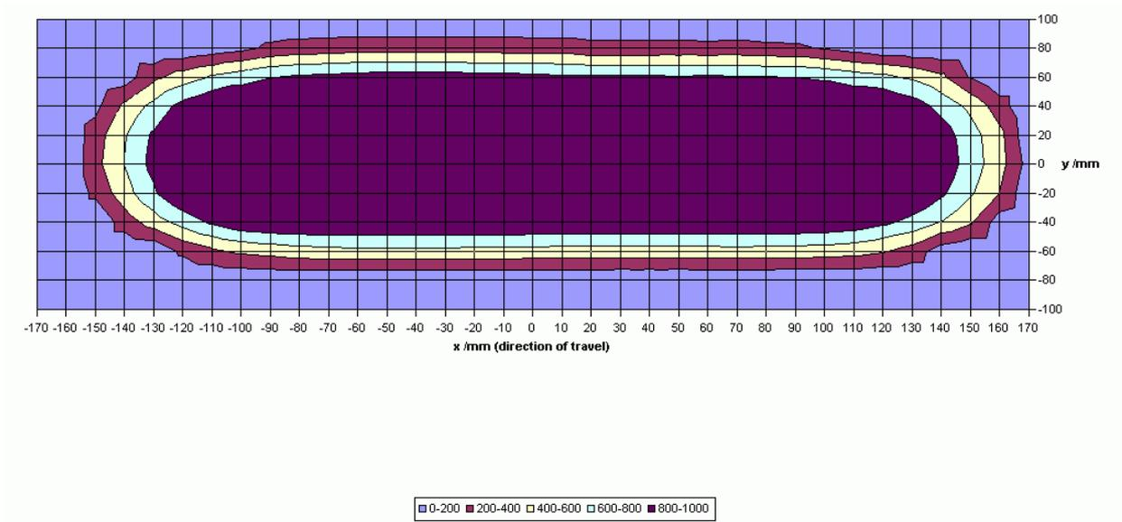
**Figure 21** Diagram 1, Reception voltage S within the antenna area at a reading distance of 40 mm
