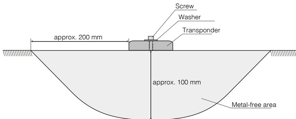
**Figure 2** Minimum iron-free area around Puck Transponder HG 70661
