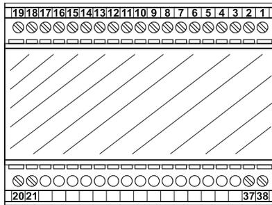
Figure 5 Outline of the interface mounting bar case
