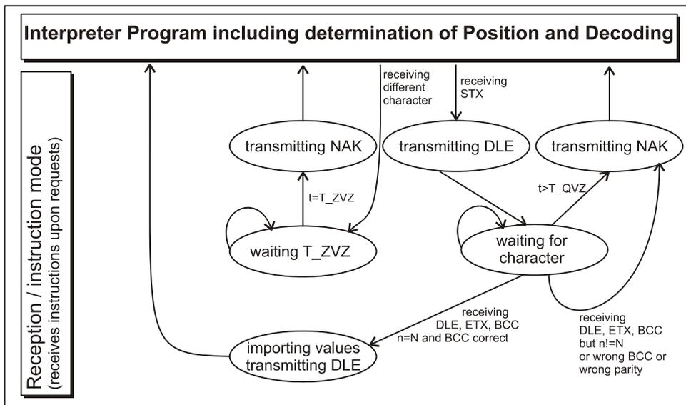
Figure 37 Status diagram procedure 3964R; PLC -> Antenna
