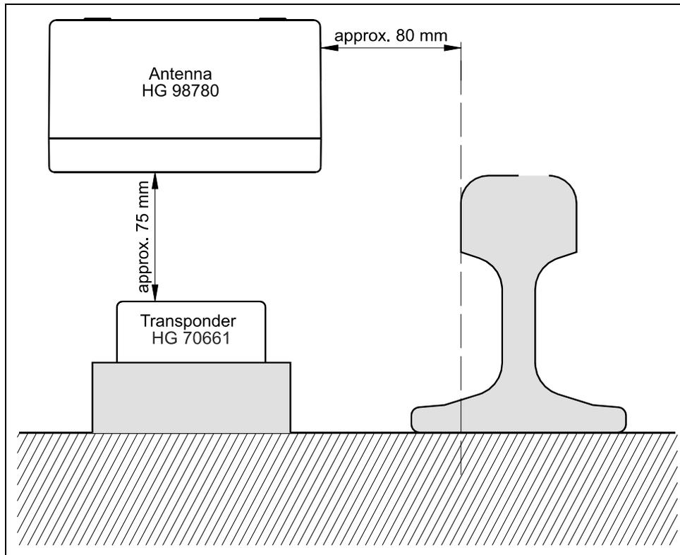
**Figure 35** Recommended distances to massive metal structures
