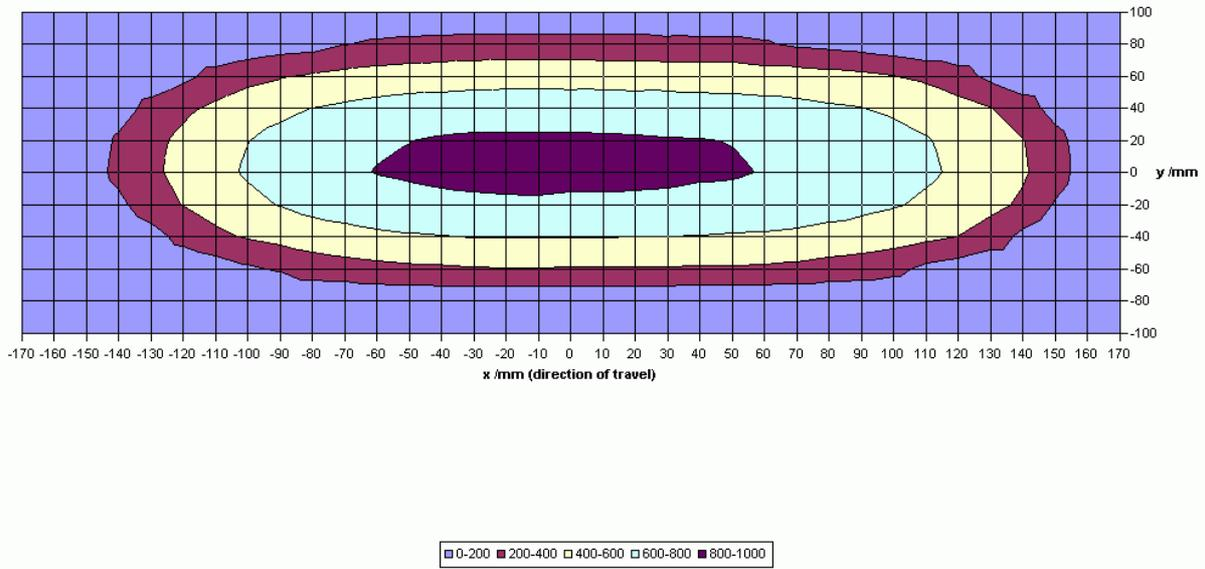
**Figure 23** Diagram 3, Reception voltage S within the antenna area at reading distance 80 mm
