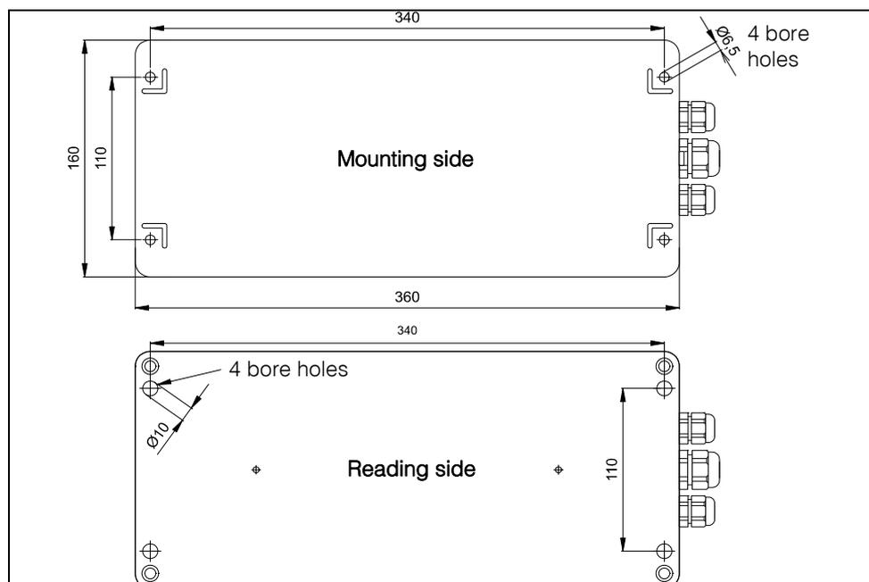
**Figure 4** Position of the mounting holes
