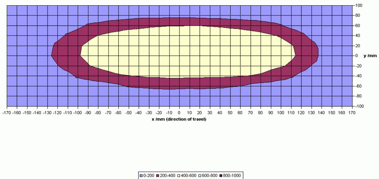
**Figure 24** Diagram 4, Reception voltage S within the antenna area at reading distance 100 mm
