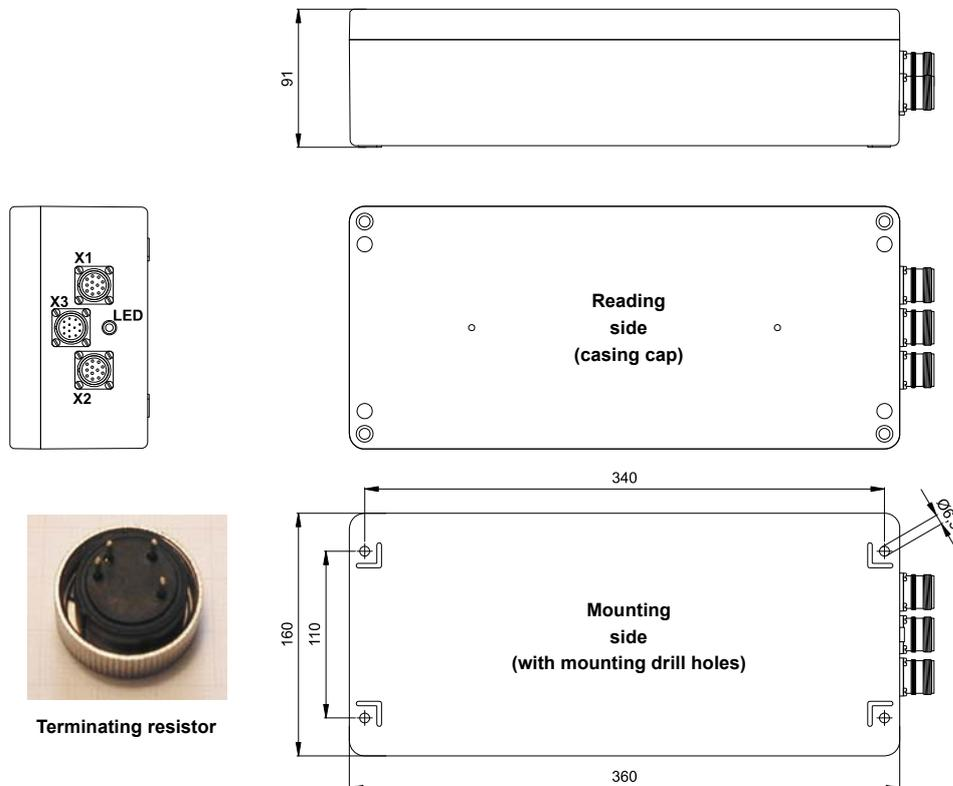
**Figure 8** Outline of antenna HG 98780YA/XA (including housing dimensions and picture of the terminating resistor / Terminator)
