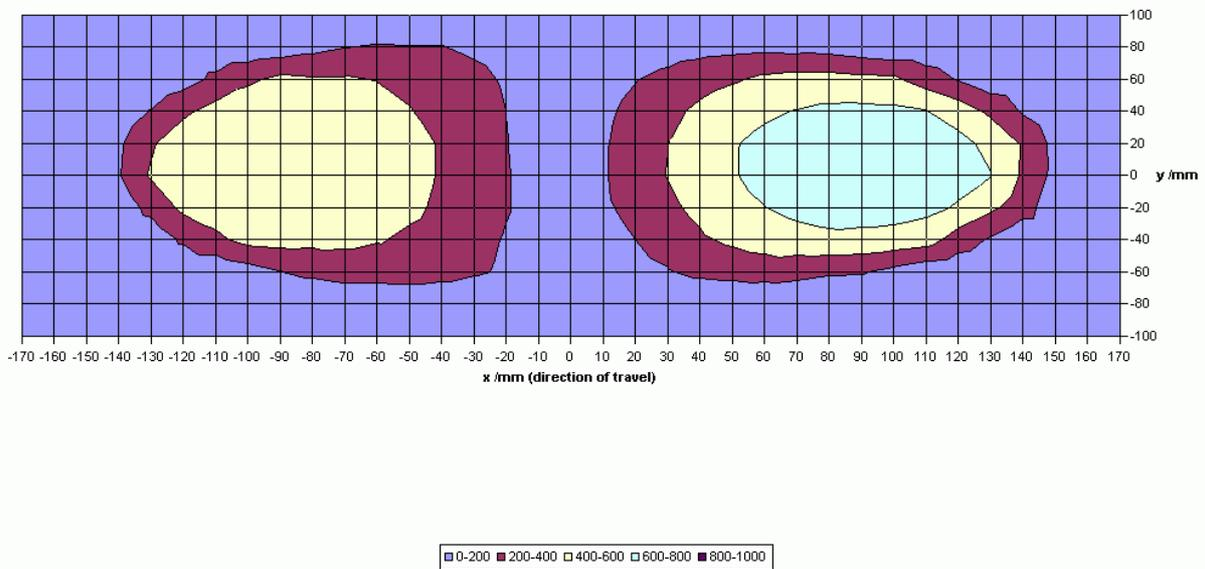
**Figure 26** Diagram 6, Reception voltage X within the antenna area at reading distance 100 mm
