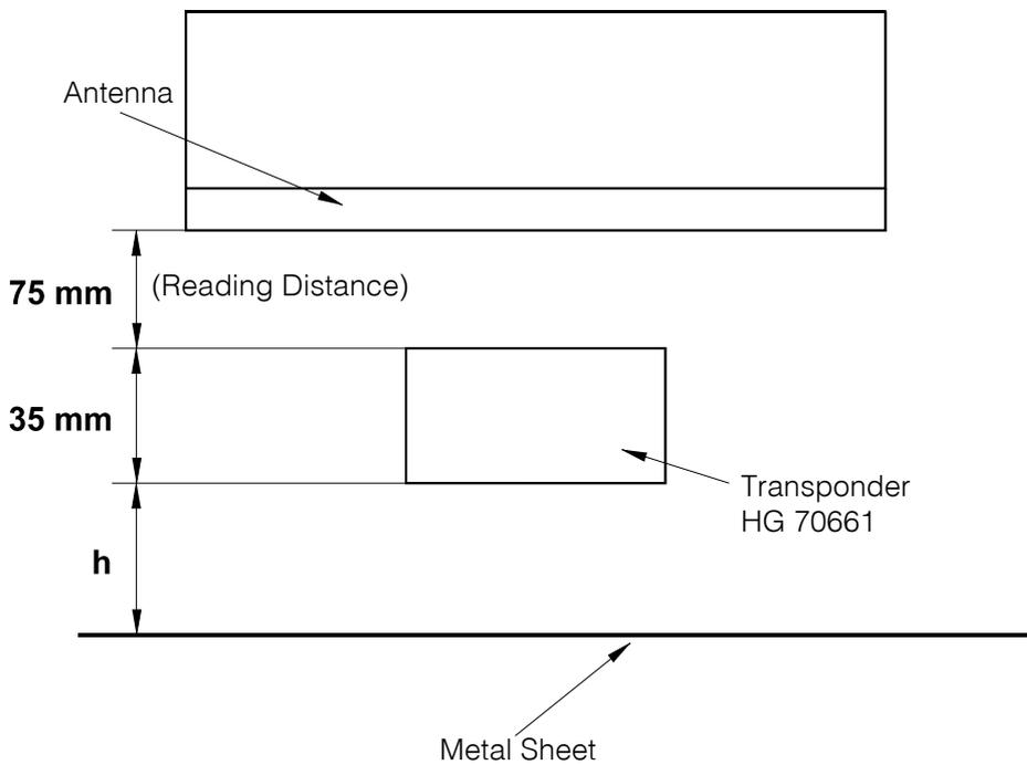
Figure 32 Attenuation of the reception level caused by metal
