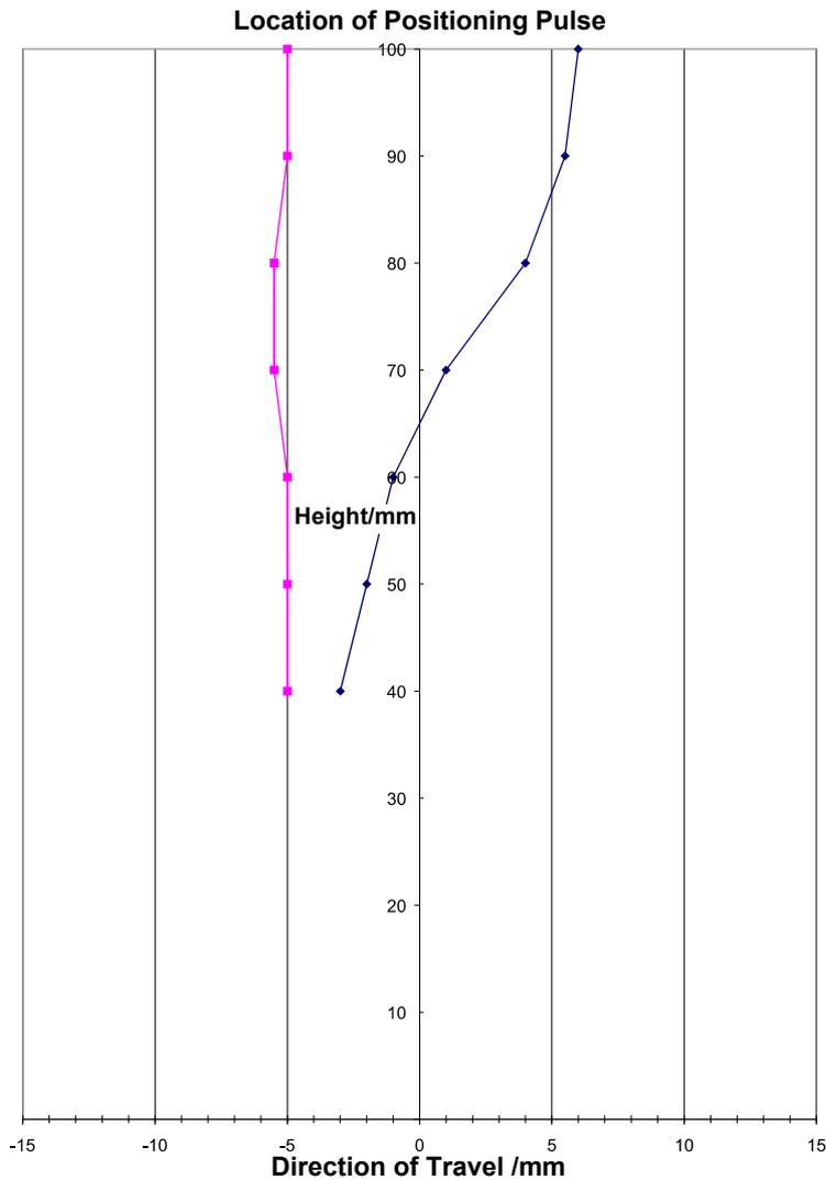
**Figure 31** Diagram 5, Location of the generation of the Posipulse on the center axis at different reading distances
