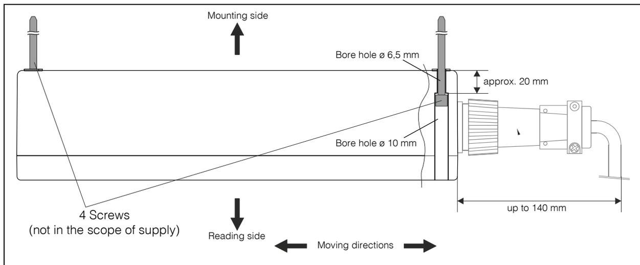
**Figure 3** Mounting the antenna
