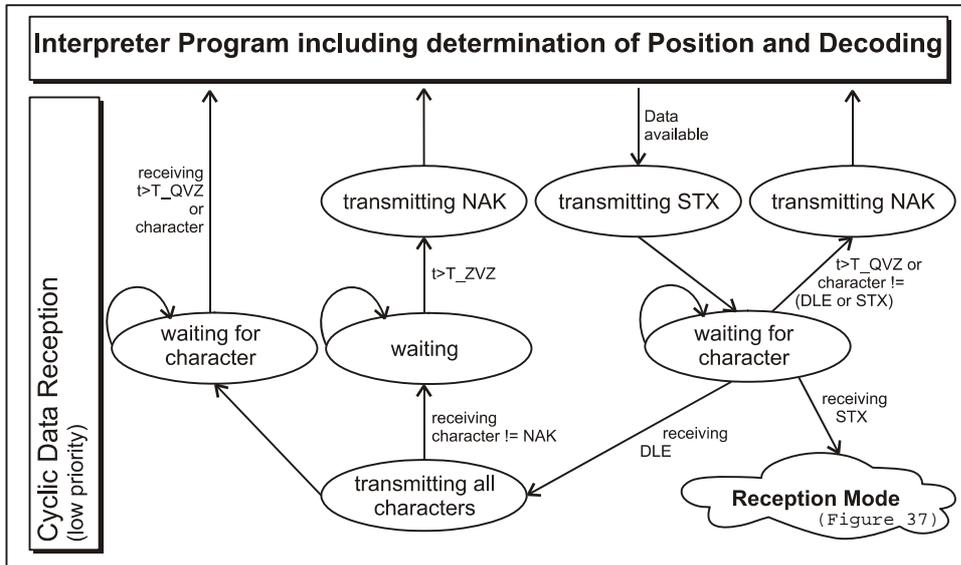
Figure 36 Status diagram procedure 3964R; Antenna -> PLC
