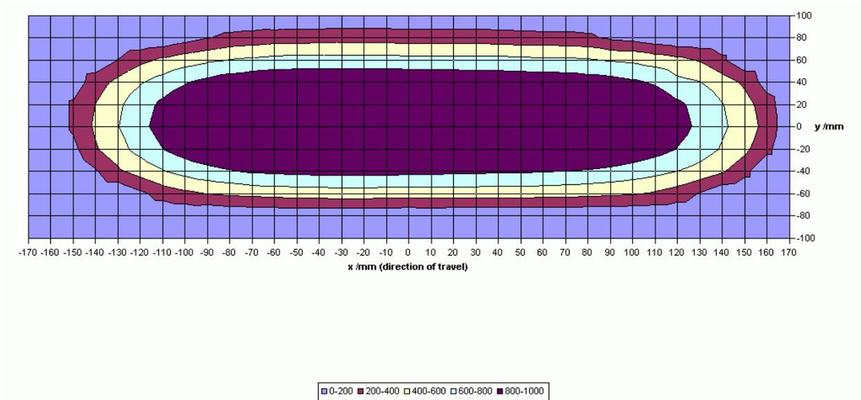
**Figure 22** Diagram 2, Reception voltage S within the antenna area at reading distance 60 mm
