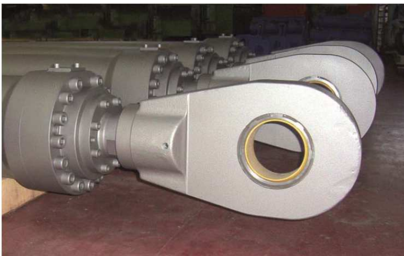
Cylinder with spherical bearing and Rod end
