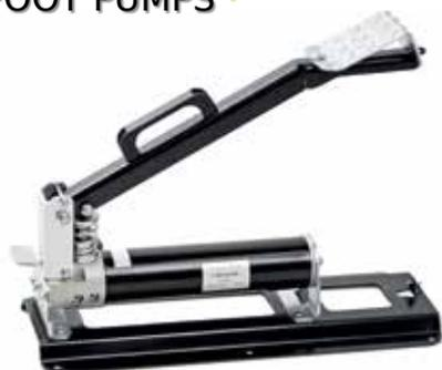
Pumps for systems and tasks where free hands of the operator are necessary. Dedicated to single-acting cylinders (FPME) or to work with special tools (e.g. nut cutters) at high pressure (F-HFP25 - two-stage pump). Equipped with own oil tank.
