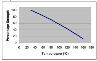
The temperature resistance test was carried out by curing the product between 2 steel lap shears. The test pieces where then left at the test temperature for 1 hour. A lap shear strength test was then performed on each sample.
