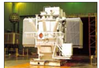
66kV 20MVA Transformer Tokyo Electric Power Company in Japan
