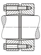
Inkofix-tension set ISH is for transmission of medium torque with regular concentricity.
