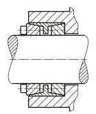
Inkofix-shrink ring ISR and Inkofix-shrink disc ISS are for efficient clamping of shafts and hubs.
