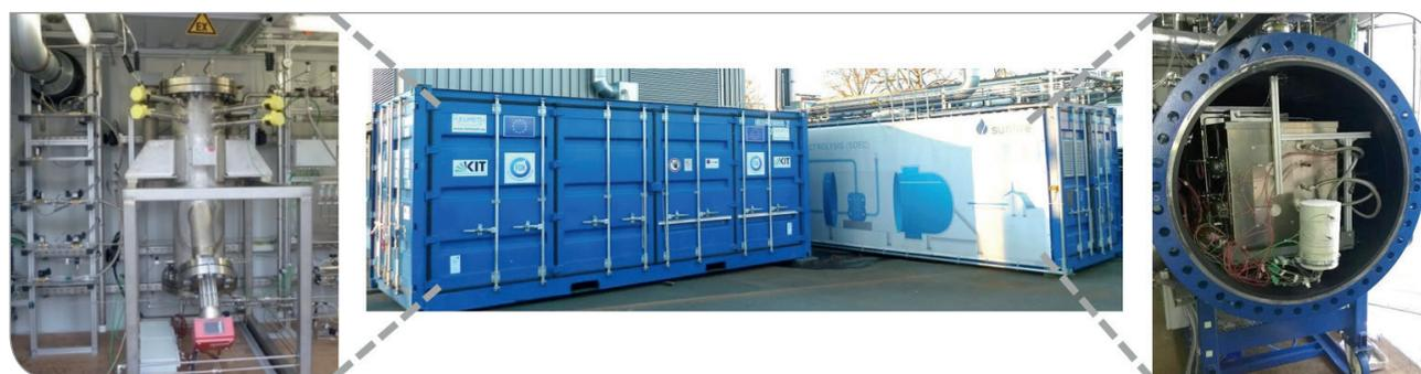
Prototype consisting of the methanation module (container on the left) and the electrolysis module (container on the right)
