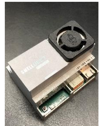
The smelldect demonstrator rapidly and easily acquires olfactory information. (Photo: Martin Sommer, KIT)
