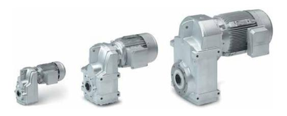
Our slimline shaft-mounted helical gearboxes are characterised by high permissible radial forces, closely stepped ratios and a low backlash. They are available in 2-stage and 3-stage designs with a maximum torque of 19,000 Nm and ratios of up to i=500 depending on your individual requirements.
