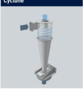
The airstream carrying fine particles enters the cyclone (centrifugal separator) tangentially at the top. The solids are carried to the outside by the rotating centrifugal airflow and pass spirally either to the collecting container or to the dust compactor mounted underneath
