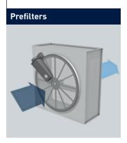
The airstream carrying coarse particles passes through a filter media. The mesh size can be adjusted to the particle size. The filter media is cleaned with continuous suction.
