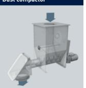
The material previously separated is picked up by a horizontal compacting screw and discharged. An agitator ensures an even feed to the screw and prevents clogging. The material is compacted by a metal spring diaphragm.
