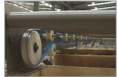
Suitable for tangential live roller drives
