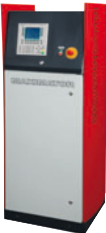
Gas proportioning Station
