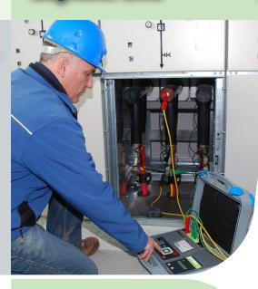
MI 3210 TeraOhm XA 10kV is a portable, battery or mains powered test instrument with excellent IP protection (IP65), intended for diagnosing of Insulation Resistance by using high DC test voltages of up to 10 kV. Because of its robustness (CAT IV protection) and high immunity to radiated RF fields it is best suited for industrial environment.
