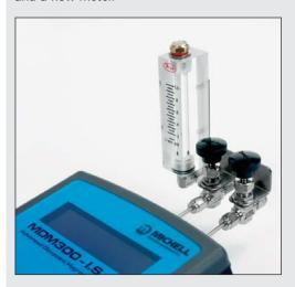
The Compressed Air Kit has a similar configuration to the Easi-fit Kit, but with the addition of a particulate filter and Rp ¼" fitting, commonly found in the compressed air industry. The fitting is connected to the filter inlet by a 2m length of PTFE tube, to allow for flexibility when coupling directly to compressed air systems.
