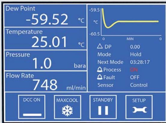
A pair of adjustable isolated alarm contacts allow the S8000 Integrale Chilled Mirror Hygrometer to be used for direct process control. A high-contrast touch screen LCD display provides entirely customizable local indication of the measured values, along with a trend graph and fault warnings.
