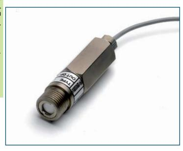
The SF Series of Dew Point Transmitters from Michell Instruments can provide 4–20mA or voltage signal for either dew point or absolute humidity with excellent accuracy and linearity. The robust housing, together with an operating pressure of up to 20 barg, makes the SF Series ideal for many dew point and moisture measurement applications.
