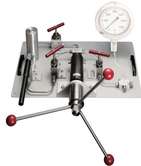
Hand pump system
