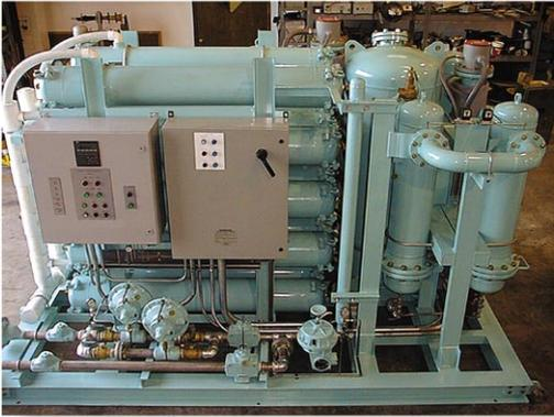
To produce Nitrogen and Oxygen, IGS Italy uses the principles of air separation. Hollow Fiber Membrane technology is used to produce Nitrogen, PSA (Pressure Swing Adsorption) technology for the production of Oxygen or high-purity Nitrogen.
