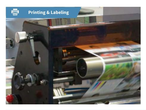
Sensitive products can be printed more quickly using linear motor technology, because the printing process is performed using position, speed, and force control. The force impacts associated with pneumatic solutions do not occur.
