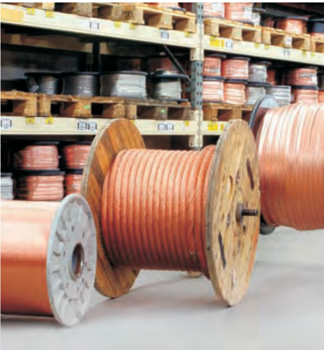
Finished products: Round stranded copper cables, braided copper tapes
