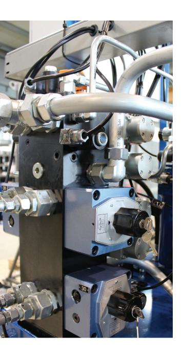
Our offer includes two major groups of flow control valves: throttle valves and flow control elements, designed for various types of mounting.
