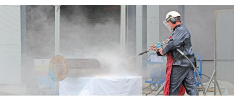
FEEDERbox is a pneumatic lance feeder (available also in electronic version) used for cleaning heat exchangers, e.g. in power plants, heat and power plants, and in petrochemical plants.
