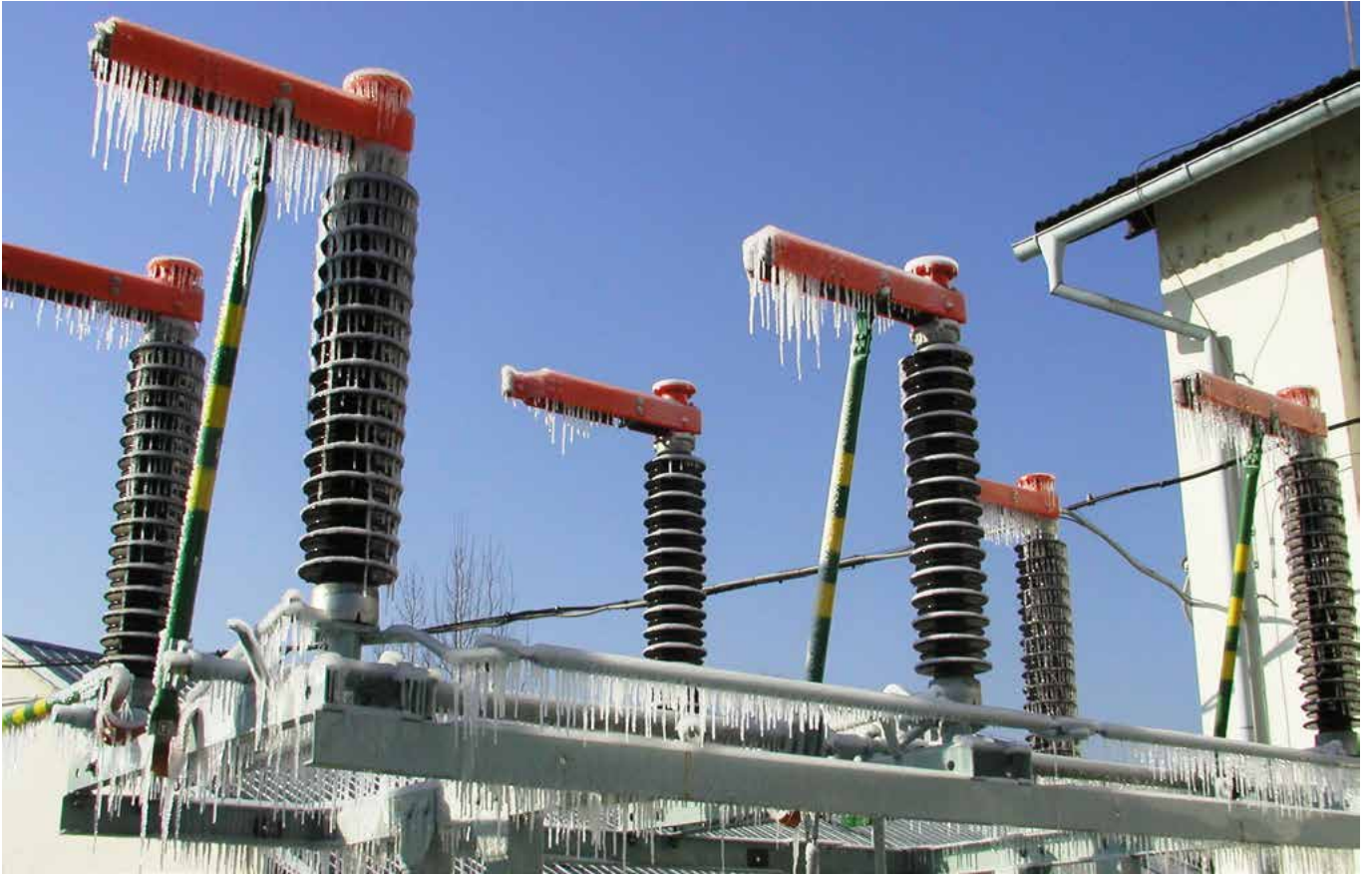
123kV Horizontal disconnectors with earthing switch during climatic test
