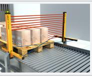
Access control for palletizers with different muting logic: T with crossed beams, L with crossed beams and T with 4 parallel beams (sequential logic with contemporaneity).
