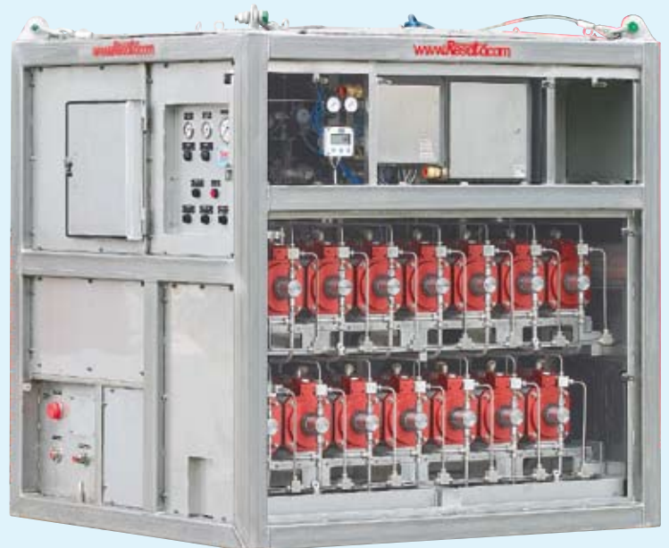
Mobile multi pump injection unit
