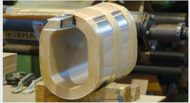
sturdy, suitable to withstand possible electrodynamic stresses caused by a short circuit.
