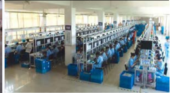
MCBs assembly lines
