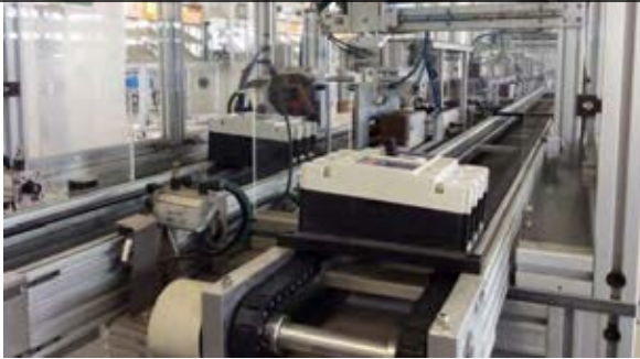
MCCBs assembly lines
