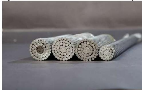
All the wires have the same nominal diameter. Most common constructions consist of 7, 19, 37 and 61 wires
